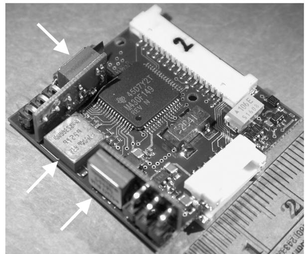
Fig. 5. Prosthesis circuitry. Arrows=rotational accelerometers, two of which are on boards perpendicular to the mother board. Scale = cm
