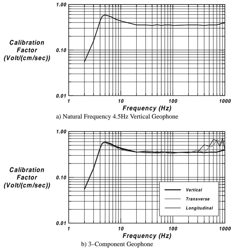
Fig. 1. Calibration curve for 4.5 Hz geophone and 3-component geophone: (a) Natural frequency 4.5 Hz vertical geophone; and (b) 3-component geophone.
