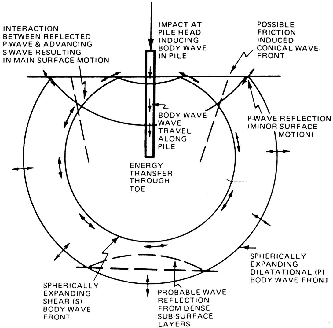
Fig. 11. Possible wavefronts from a driven pile [13].
