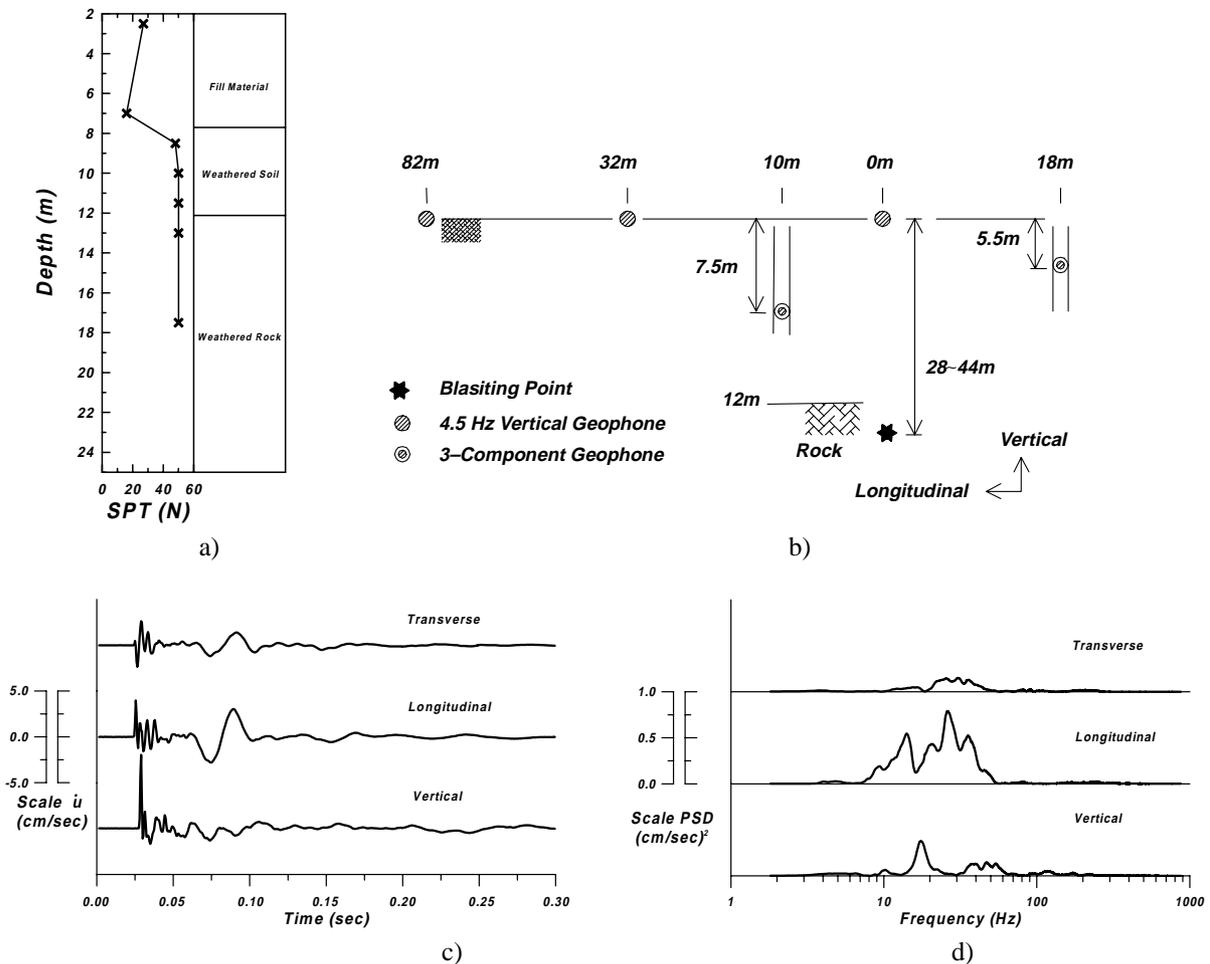
Fig. 3. Site information, typical 3-component time records and power spectral density induced by in-depth blasting. (Charge weight: 2 kg TNT; depth of explosion: 28 m, recorded at distance 10 m, 7.5 m, horizontal and depth, respectively.)
