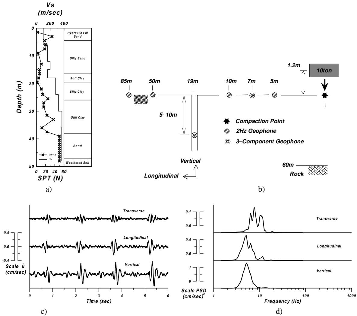
Fig. 5. Site information, typical 3-component time records and power spectral density induced by hydraulic hammer compaction. (Recorded at horizontal distance 7 m.)
