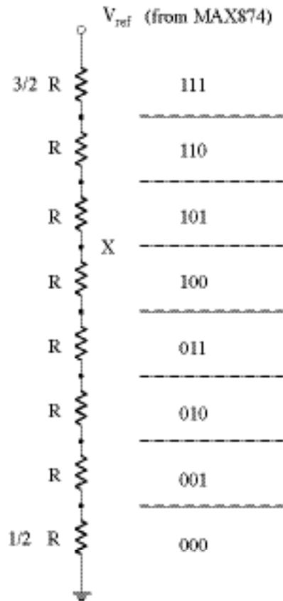
Figure 1: Voltage divider circuit with digital voltage “bins.” A flash analog-to-digital converter determines whether an input voltage lies between two adjacent node voltages in the resistor divider chain. The corresponding bin has a digital assignment.
